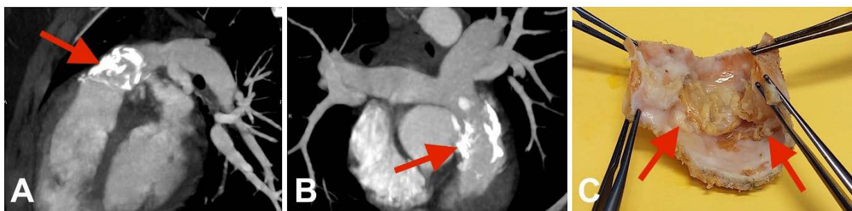
Fig. 1. Calcified glutaraldehyde-treated bovine jugular vein conduit, 9 years after implantation for RVOT reconstruction (Ross procedure): A, B – CT images; C – macrophotograph of the explanted conduit. Red arrows indicate large calcium deposits in the conduit wall and leaflets (data sourced from the archive of the Meshalkin National Medical Research Center)
